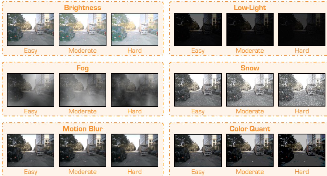
Figure 7: Visualizations of different Camera sensor corruptions under three severity levels, i.e. , Easy, Moderate, and Hard, in our benchmark. Best viewed in color and zoomed in for details.
